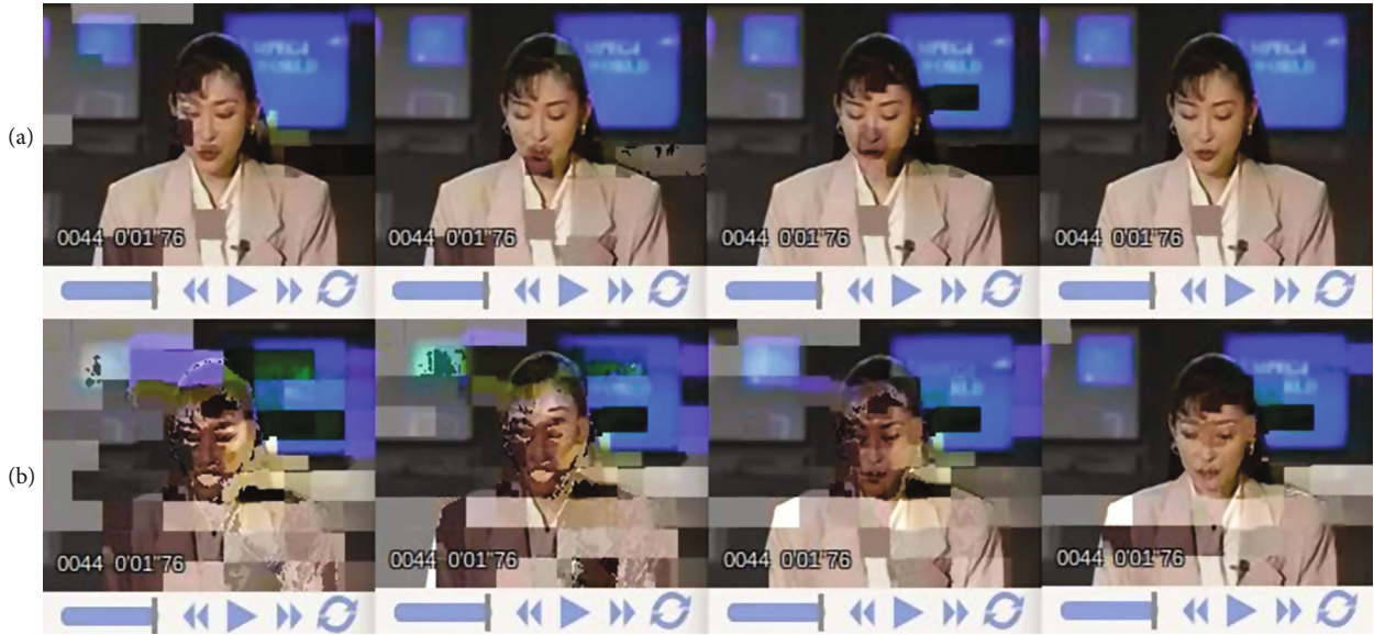
FIGURE 7: Subjective video quality performance of the Akiyo sequence frame using the proposed system (a) and DSTS-SP RSC scheme (b) summarized in Table 2 at E_b/N_0 values of (1, 2, 3, 4) dB (left to right).
